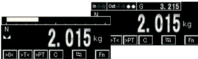
Version T – Clavier, Bargraphe et barre d'état T version – Keyboard, Bargraph and status bar
